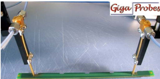
Fig. 1) Two GigaProbes™ connected through SMA cables and to the TDR heads are used to acquire the differential Reference (Open), TDR, TDT Waveforms and ported into IConnect® for processing.
