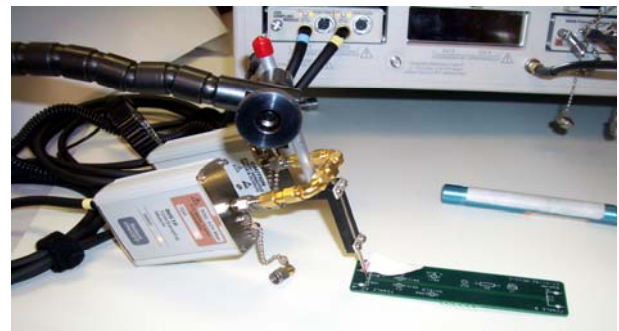
Fig 2) For a faster TDR pulse, remove the cable and directly connect the GigaProbes™ directly to the TD sampling head via a high speed coupler.
