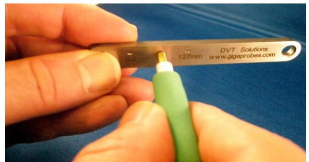
Fig. 3) Signal - Signal Pitch Calibration (patent pending) - Place the probe tips in the Model 10 SMA stainless steel calibration wrench adjusts S - S pitch to a fixed 0.8 mm, 1.0 mm, or 1.27 mm spacing. Use the Desk-Top Macro-lens Inspection Station to view probe tips, probing location and the precision Stainless Steel Tweezers for fine pitch adjustments.
