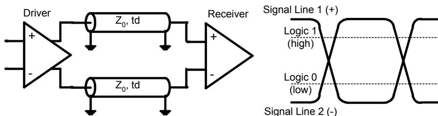
**Figure 1. Differential signaling. Two signals are used to transmit a single bit of data from the driver to the receiver. When the signal on one line is logical high, it is logical low on the other line, and vice versa.**
