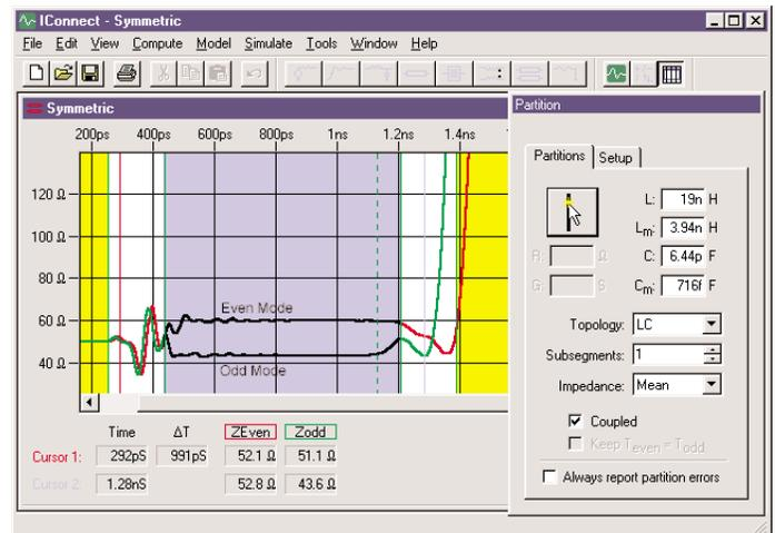
**Figure 9. Applying the even and odd analysis to compute L-C matrices for the coupled lines in IConnect software. Note that for long lines a large numbers of subsegments must be used to accurately model the line**
