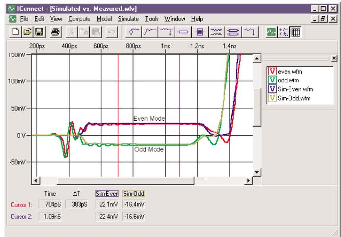
**Figure 8. Verifying the differential line model in IConnect software. Simulations with both even and odd mode stimuli are performed using an integrated interface to a SPICE simulator and the simulation results are compared to the measurement data**
