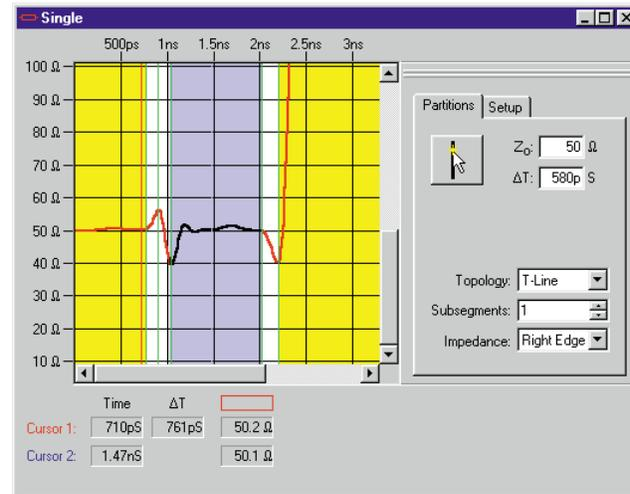
**Figure 3. DUT interface board impedance profile. The impedance profile is partitioned into sections, and the equivalent SPICE model for the board is computed by IConnect TDR software**
