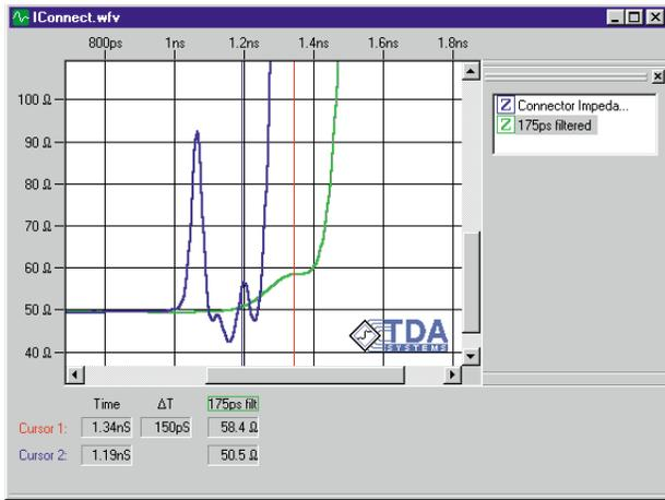
**Figure 6. Impedance profile of a connector filtered at 175ps**
