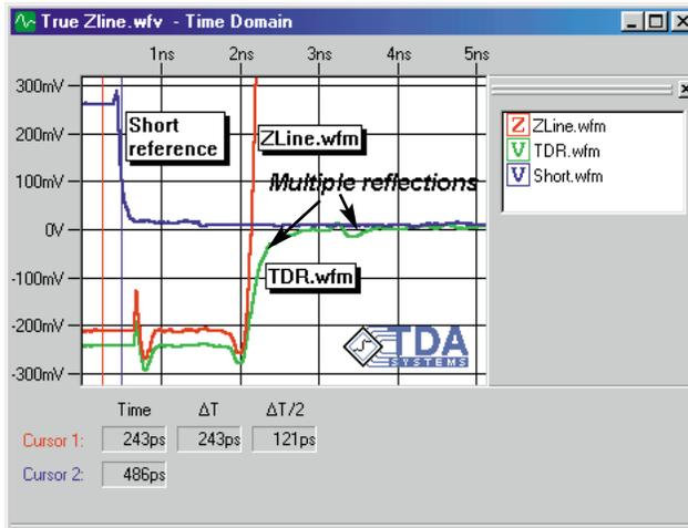
**Figure 2. Multiple reflections in the TDR waveform. The true impedance profile (ZLine) is computed in IConnect software, and allows the test engineer to extract the equivalent circuit model for the load board interconnect easily**
