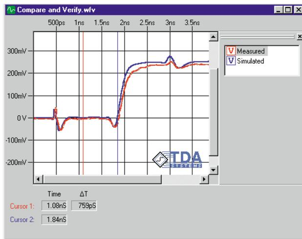
**Figure 4. Comparison of simulated and measured data for the DUT interface board. Excellent correlation is achieved even at a very fast 35-40ps TDR rise time**
