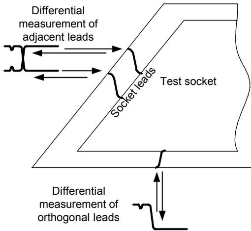
**Figure 11. Measurement setup for differential TDR characterization of an ATE socket using orthogonal differential analysis technique**
