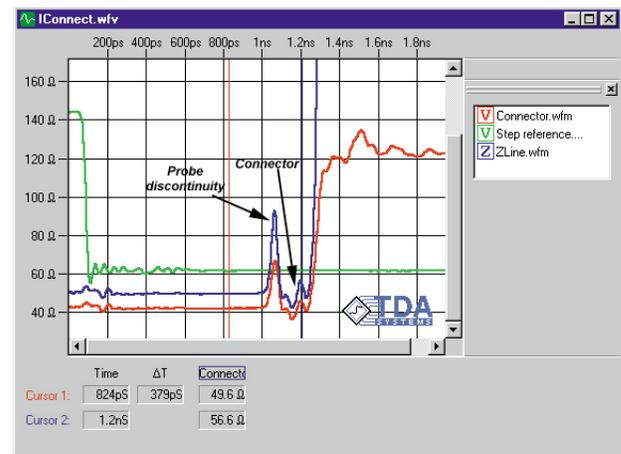
**Figure 5. Analyzing the load board connector. True impedance profile makes it easy to distinguish different segments of the connector and the fixturing used in the connector measurements**
