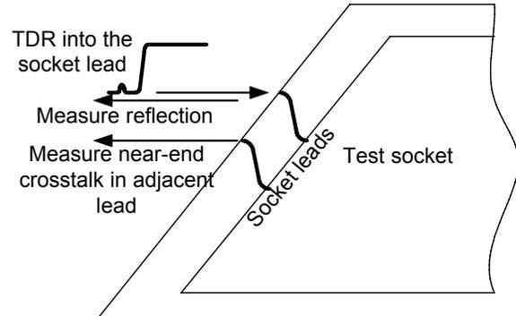
**Figure 7. Measurement setup for single-ended TDR characterization of an ATE socket. The socket leads must be shorted to ground on the inside of the socket for inductance measurements, and left open-ended for capacitance measurements**
