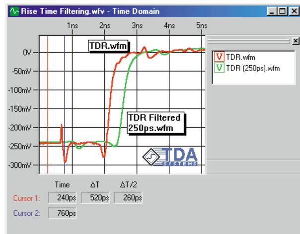
**Figure 1.** Rise time filtering is important when performing TDR characterization of the load board. At a more realistic slower rise time of 250ps, the discontinuities due to connector are not as large as they are at a 35ps TDR oscilloscope rise time
