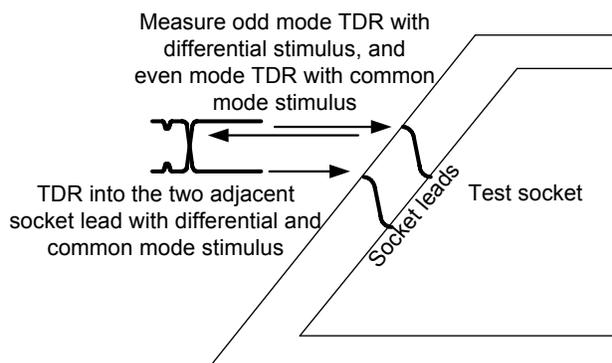
**Figure 10. Measurement setup for differential TDR characterization of an ATE socket**
