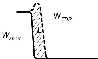
**Figure 9. Self-inductance measurement**
