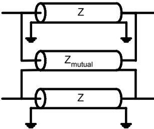
**Figure 7. Simplified differential transmission line model**
