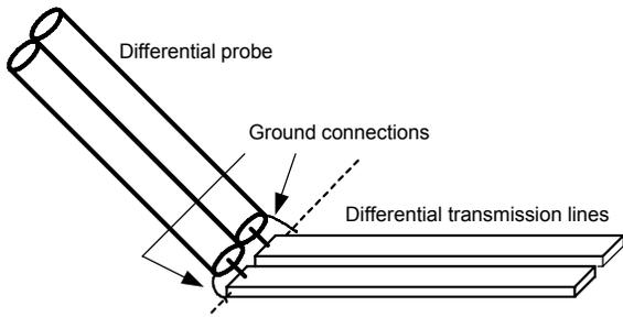
**Figure 2. Practical differential TDR probe and measurement setup**
