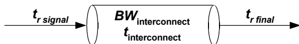
Figure 1. Rise time degradation is the result of limited bandwidth in the lossy interconnects
